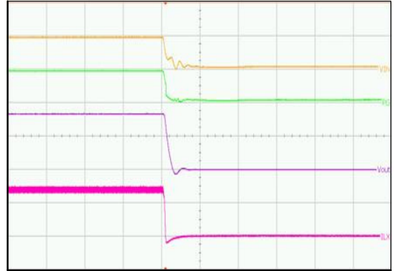
(VIN = 5 V, VOUT = 1.8 V, IOUT = 3 A) Upper Trace: Input Voltage, 5 V / div Second Trace: Power Good Pin Voltage, 5 V / div Third Trace: Output Voltage, 2 V / div Lower Trace: Inductor Current, 2 A / div Time = 200 \mu s / div
