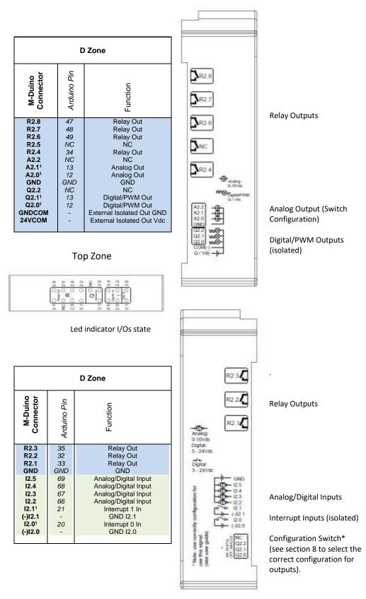
See section 8 to select suitable switch configuration for enable these connections.
