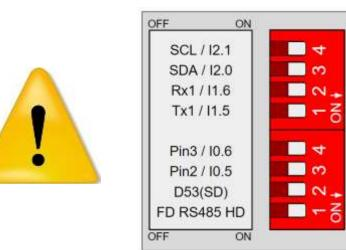
**4. SCL/I2.1:** Choosing between SCL or the input I2.1. If this switch is ON, it enables the I2.1 input and disables the SCL. If this switch is OFF, it enables SCL and disables I2.1.
