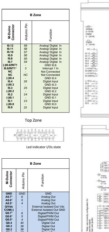
Configuration Switch\* (see section 8 to select the correct configuration for outputs). Analog Outputs Voltage Supply/Reference for Digital/PWM Outputs (isolated) PWM/Digital Outputs
