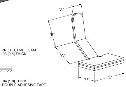
NOTES: 1. MATERIAL: ALUMINUM (RMS-194). 2. POLYETHYLENE ADHESIVE FOAM TAPE (RMS-93). 3. POLYETHYLENE FOAM COATING (RMS-264).
