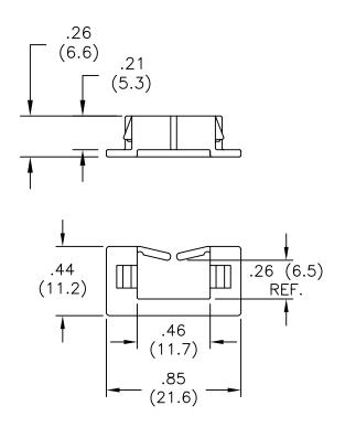
RECOMMENDED INSTALLATION PANEL THICKNESS RANGE: .032 TO .079 (0.8 TO 2.0)
