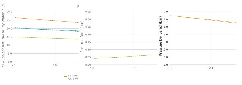
\*  $\Delta T$  (Coolant Outlet - Facility Water In) is the temperature difference between the facility water temperature and the coolant temperature that is at the outlet of the heat exchanger during steady-state operation. This temperature difference would initially be 0 and increase to the steady state value under load. This would also be the temperature at the inlet to the application.
