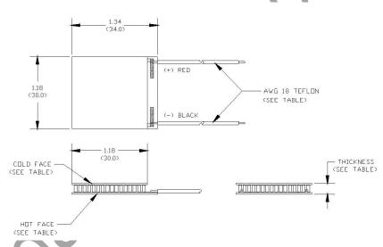
Ceramic Material: Alumina (Al<sub>2</sub>O<sub>3</sub>) Solder Construction: 271°C, Proprietary
