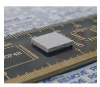
Laird's Tflex™ HD7.5 gap filler is a new developed very soft silicone material in our high deflection series. With a thermal conductivity of 7.5W/ mk, Tflex™ HD7.5 is designed to provide superior pressure versus deflection characteristics. The material will provide minimal stress on components during application while maintaining low thermal resistance. As a result, less mechanical and thermal stresses will be experienced within your device.
