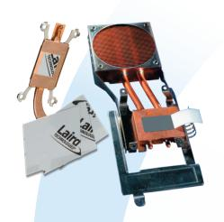
Tpcm<sup>™</sup> 900 is a high performance, non-electrically conductive phasechange material. At 50°C, Tpcm<sup>™</sup> 900 begins to soften and flow, filling the microscopic irregularities of both the thermal solution andthe component's surfaces, thereby reducing thermal resistance. It is a flexible solid at room temperature and freestandingwithout reinforcing components that reduce thermal performance.
