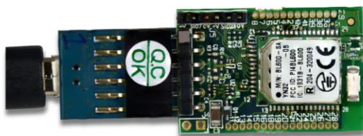
Figure 19: BA600-0x connected to the USB-UART bridge board
