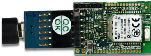
Figure 19: BA600-0x connected to the USB-UART bridge board
