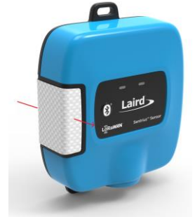
Figure 8: Air flow through sensor
