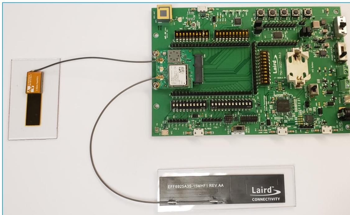
Figure 8: External antenna attachment for 453-00011 Pinnacle™ 100 modem
