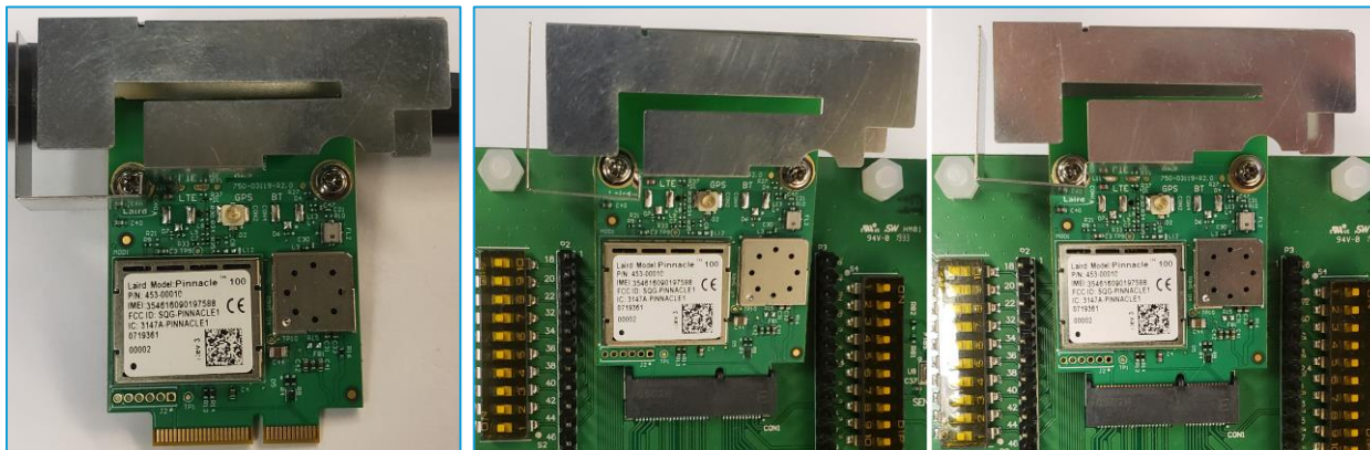
Figure 7: Attaching a 453-00010 Pinnacle™ 100 modem to a DVK
