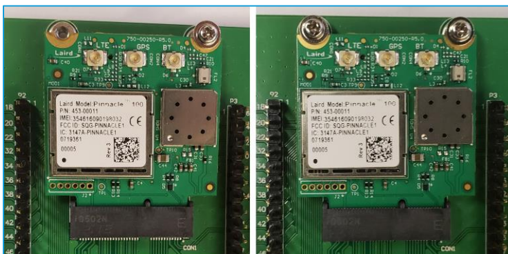
Figure 6: Attaching a 453-00011 Pinnacle™ 100 modem to a DVK
