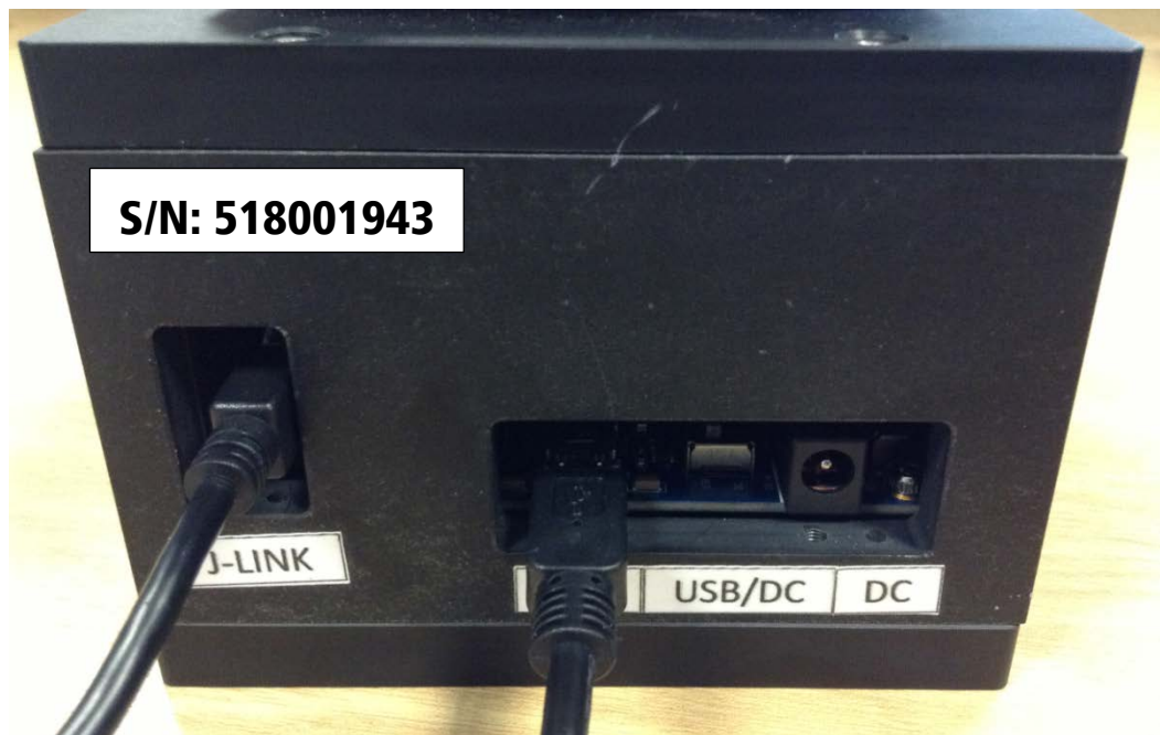
Figure 7: J-LINK cable connecting to programming jig
