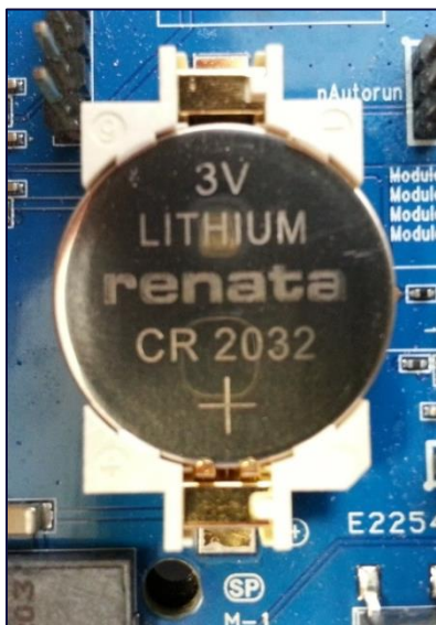
Figure 21: Inserting the coin cell (step 2)
