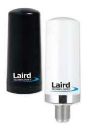
Laird's unique Phantom antenna operates simultaneously in the 806-896 MHz, 1850-1990 MHz, and 2500-2700 MHz bands. The mechanically robust design is suitable for both indoor and outdoor applications. With wide bandwidth and a low angle radiation pattern that is superior to traditional gain antennas in most applications, the antenna can be used in both ceiling mount and surface mount applications.
