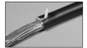
4.03 Place terminal wrench over stud and push down to bend corners and pull slit together.
