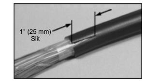
Slit web approximately 91" (2.3 m) on self-supporting cable 20" 48' Cable Support (1219mm) (510mm) Spacer 2" (50mm) (50mm) lo" ⇒ 10' (250mm) (250mm) Lashed cable support and spacer (use appropriate size of cable spacer to keep cable at the same level or slightly lower that the end seal openings) Trim Core Wrap to extend approximately 1" (25mm) past the outer sheath. If core wrap is damaged, wrap with vinyl tape.
