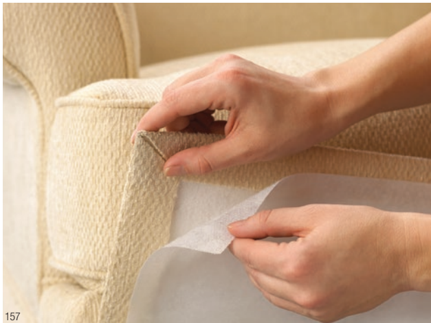
These solvent and water based adhesives are often used as a “third hand” to hold lightweight materials in place until they can be sewn or held in place by other assembly methods.
