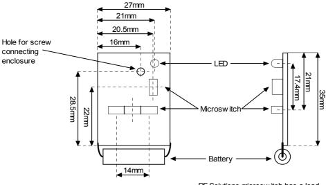
RF Solutions microswitch has a lead pitch of 6.35mm and a height of 4mm
