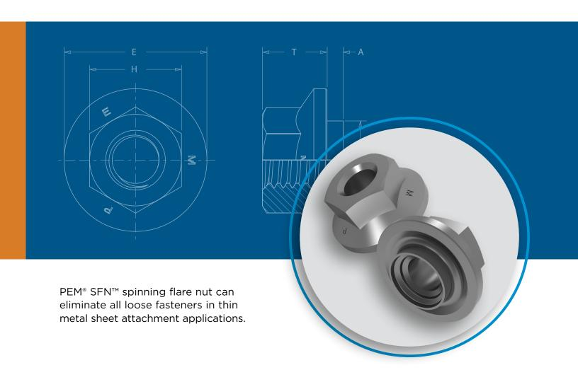
PEM® SFN™ spinning flare nuts are installed by simply pressing them into a properly sized, pre punched mounting hole. These fasteners are then permanently captivated in the panel but still able to spin freely within the sheet. This allows quick attachment of mating hardware, eliminating much of the need for loose fasteners such as flange nuts. When used with a self-clinching stud or other externally threaded fixed hardware, all loose hardware is eliminated from the applications.
