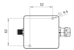
Mounting holes in the aluminum housing are accessible on removal of the lid.
