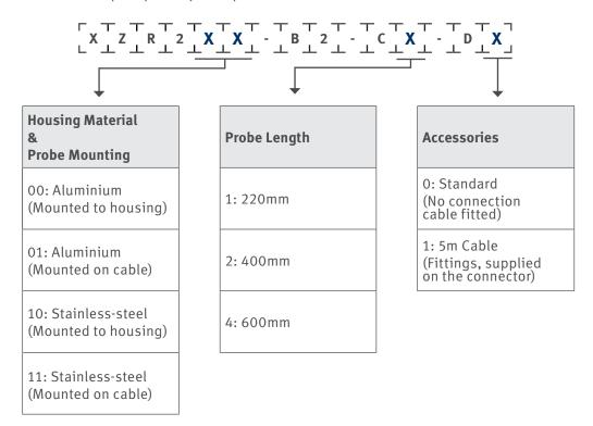
For example, if you require a transmitter in a stainless steel housing with a 600mm probe length and 5m cable, you would order: XZR210-B2-C4-D1
