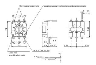
Unless otherwise specified, tolerance: ± 0.3 (Unit: mm)
