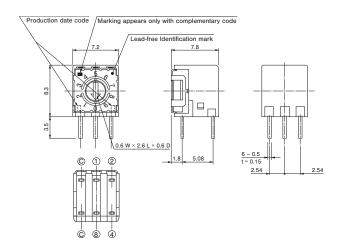
Unless otherwise specified, tolerance: ± 0.3 (Unit: mm)
