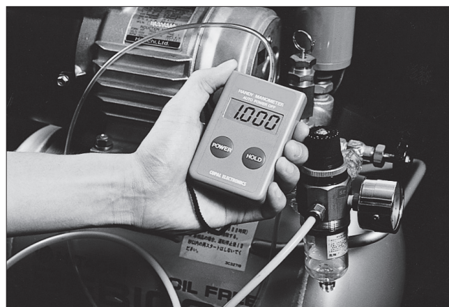
▲ Measurement of source pressure from a compressor.
