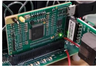
Figure 4. Green illuminated LD2 on MA330048
