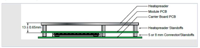
Cooling solutions provided by Kontron for compact sized Computer-on-Modules are 27 mm in height from module bottom to heatsink top.
