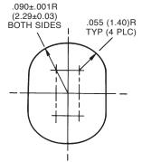
A positive mechanical detent is built into the cam rod shown here in cross section.
