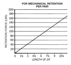
Clamping pressure is not only essential to heat transfer, but also a critical requirement for retention of PCBs under severe shock and vibration. ZIF retainers have been subjected to the most extreme test conditions specified in MIL-STD-810C.
