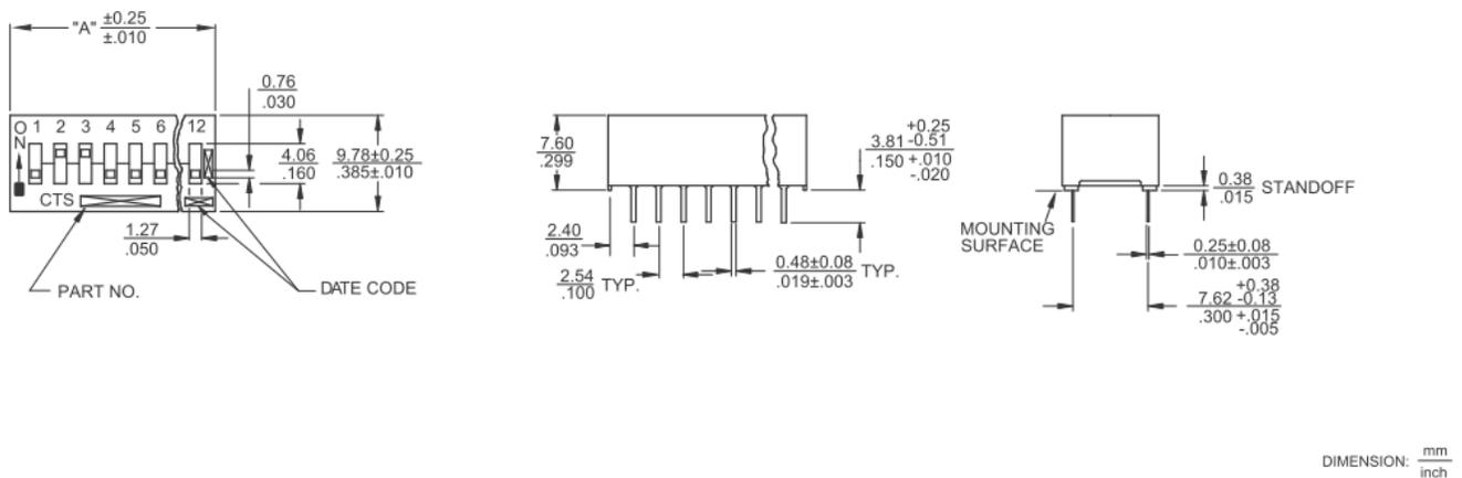
Figure 3 – Extended Actuators
