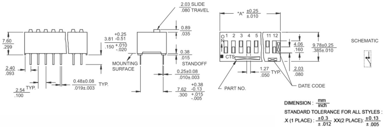
Figure 2 – Low Profile Actuators
