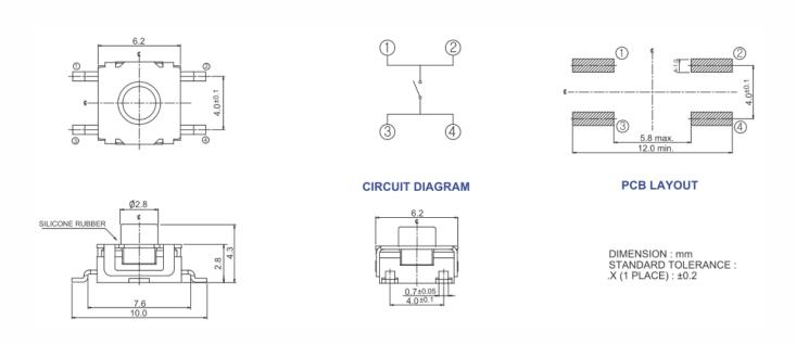
Figure 2 – 222LJV, Surface Mount J Bend, Actuator Height 4.3mm
