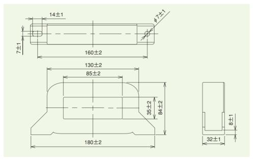
Figure 79. FT-3KL V series core
