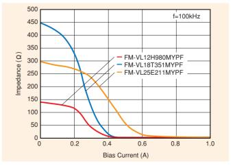
Figure 25. DC superposed charactaristics of impedance for single-phase VL coils
