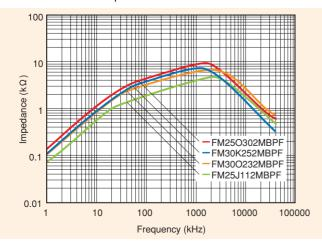
Figure 38. Frequency dependence of impedance for three-phase FM coils with rated current 25A-30A
