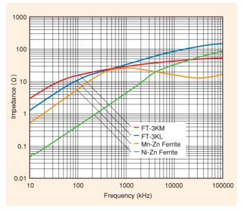
Figure 57. Frequency dependence of impedance
