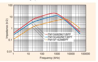
Figure 19. Frequency dependence of impedance for single-phase FM coils with rated current 15A
