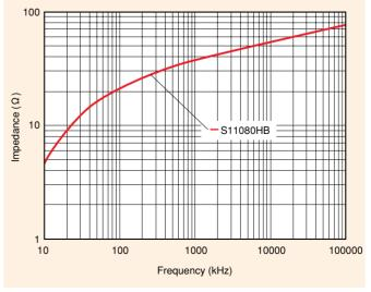
Figure 81. Frequency dependence of impedance for S11080HB
