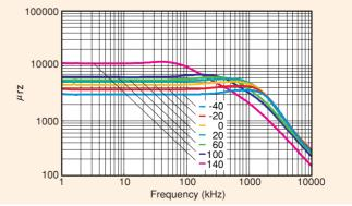
Figure 53. Temperature dependence of impedance permeability (  $\mu_{\rm TZ}$ ) for Mn-Zn ferrite
