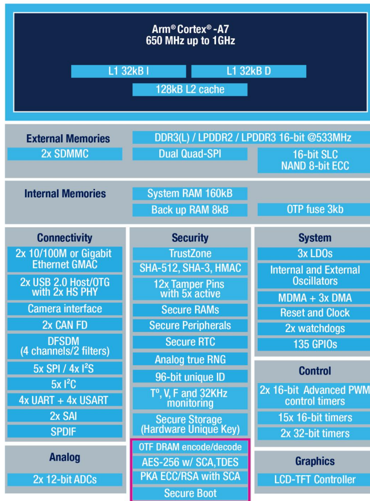
STM32MP135 Block Diagram
