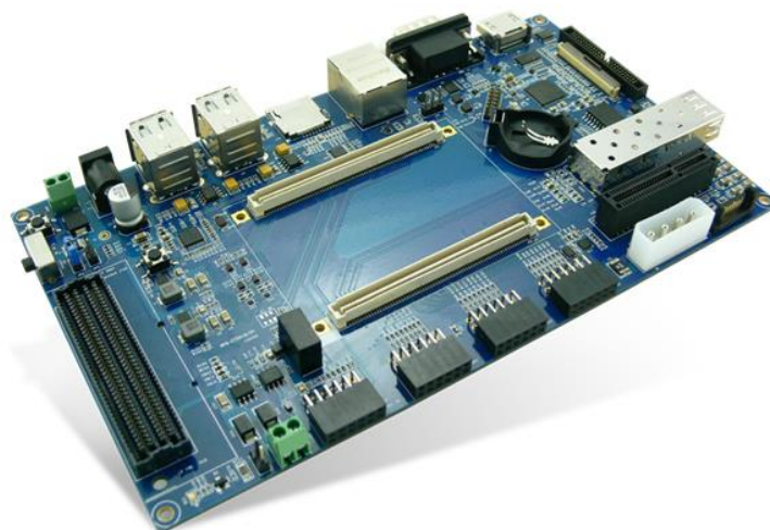
Figure 1-6 MYD-C7Z010/20 Base Board for MYC-C7Z010/20 CPU Module
