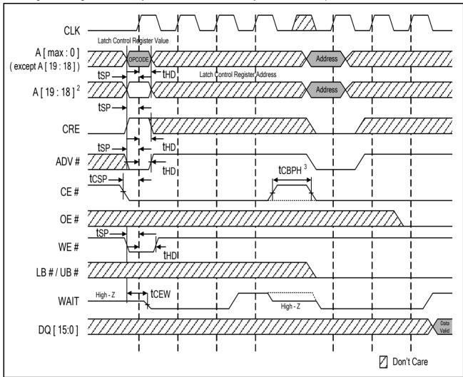
Note: 1. Non-default BCR settings for synchronous mode configuration register WRITE followed by READ ARRAY operation: Latency code 2(3 clocks); WAIT active Low; WAIT asserted during delay.
