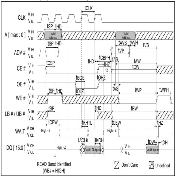
Note: 1. Non-default BCR settings for burst READ followed by asynchronous WRITE using ADV#: Fixed or variable latency; latency code 2(3 clocks); WAIT active LOW; WAIT asserted during delay.
