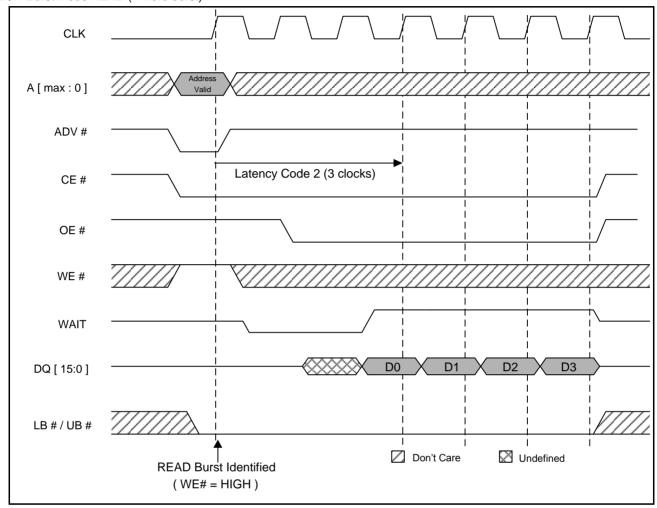
Note: Non-default BCR settings for burst mode READ (4-word burst): Fixed or variable latency; latency code 2 (3 clocks); WAIT active LOW; WAIT asserted during delay. Diagram is representative of variable latency with no refresh collision or fixedlatency access.
