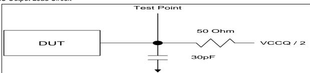
Note: All tests are performed with the outputs configured for default setting of half drive strength (BCR[5:4] = 01b).
