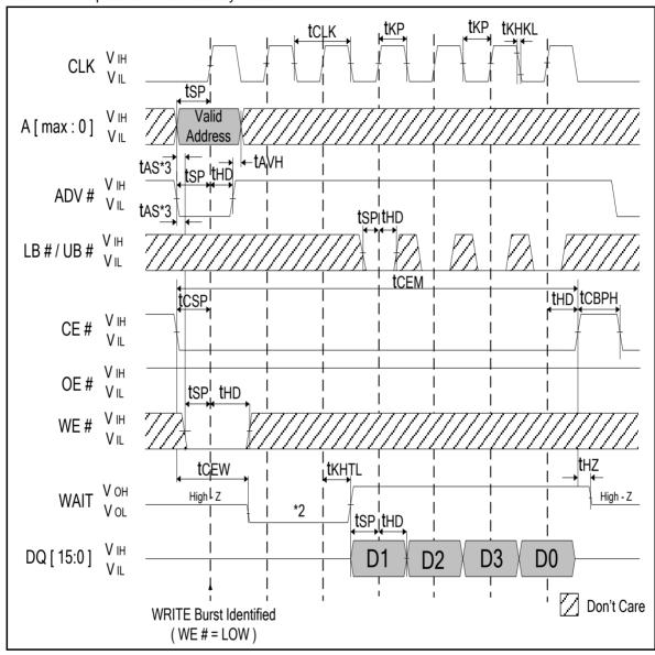
Note: 1. Non-default BCR settings for burst WRITE operation in fixed latency mode; Fixed latency, latency code 2)3 clocks); WAIT active LOW; WAIT a asserted during delay; burst length 4; burst wrap enabled.
