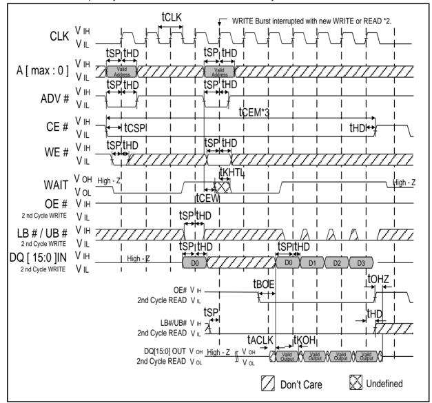
Note: 1. Non-default BCR settings for burst WRITE interrupted by burst WRITE or READ in variable latency mode: Variable latency; latency; code 2(3 clocks); WAIT active LOW; WAIT asserted during delay. All bursts shown for variable latency; no refresh collision.
