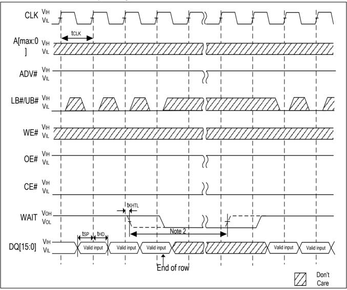
Notes: 1. Non-default BCR settings for burst WRITE at end of row: fixed or variable latency, WAIT active LOW, WAIT asserted during delay (shown as solid line).
