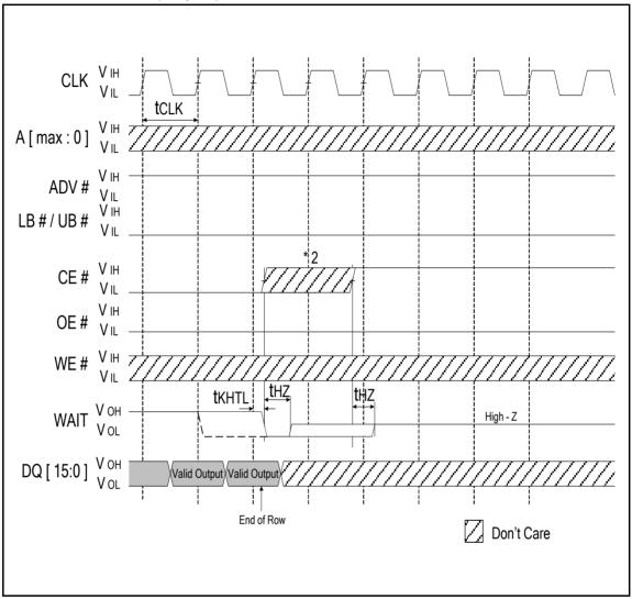
Note: 1. Non-default BCR settings for burst READ at end of row; fixed or variable latency; WAIT active LOW; WAIT asserted during delay.
