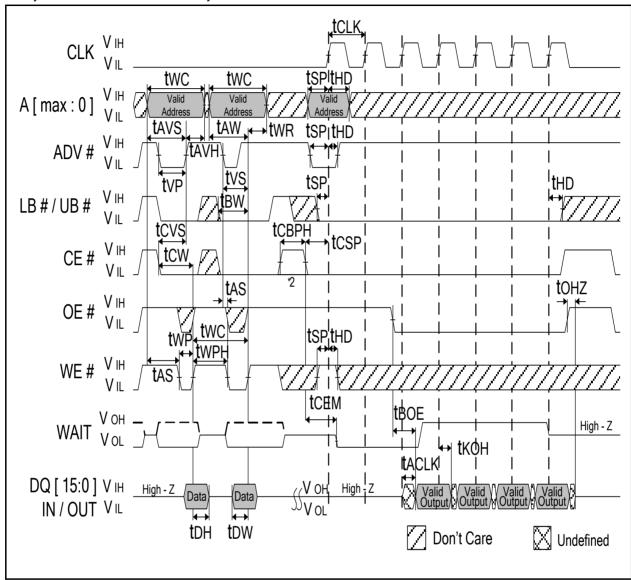
Note: 1. Non-default BCR settings for asynchronous WRITE followed by burst READ: Fixed or variable latency; latency code 2(3 clocks); WAIT active LOW; WAIT asserted during delay.
