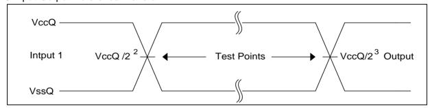
Note: 1. AC test inputs are driven at VccQ for a logic 1 and VssQ for a logic 0. Input rise and fall times (10% to 90%) <1.6ns.
