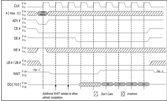
Note: Non-default BCR settings for refresh collision during variable-latency READ operation; latency code 2 (3 clocks); WAIT active LOW; WAIT asserted during delay.
