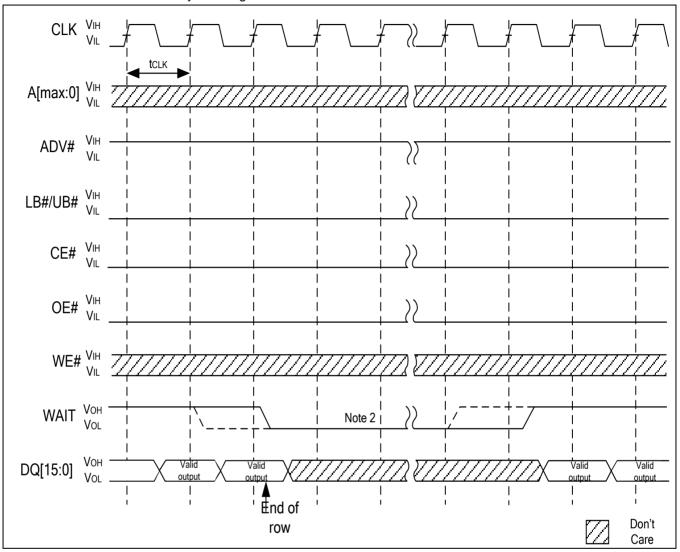
Note: 1. Non-default BCR settings for burst READ at end of row fixed or variable latency, WAIT active LOW, WAIT asserted during delay (shown as solid line).
