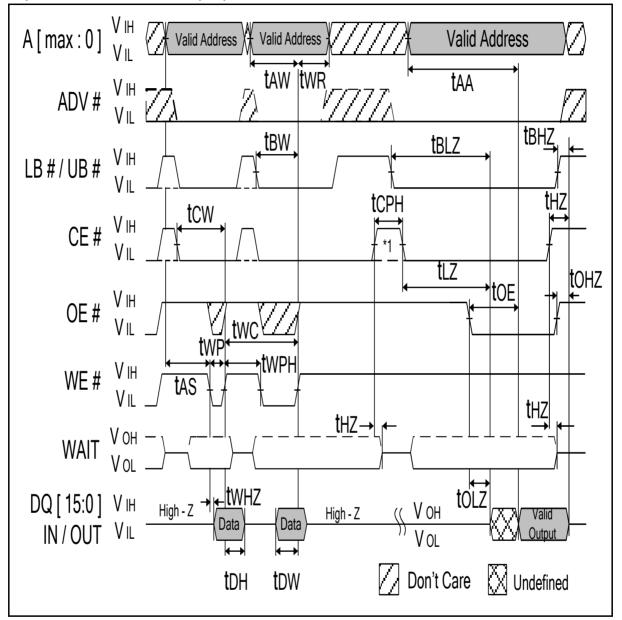
Note: 1. When configured for synchronous mode (BCR[15] = 0), CE# must remain HIGH for at least 5ns (tCPH) to schedule the appropriate refresh interval, Otherwise, tCPH is only required after CE#-controlled WRITEs.
