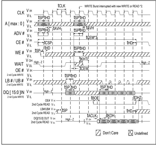
Note: 1. Non-default BCR settings for burst WRITE interrupted by burst WRITE or READ in fixed latency mode: Fixed latency; latency code 2(3 clocks); WAIT active LOW; WAIT asserted during delay.
