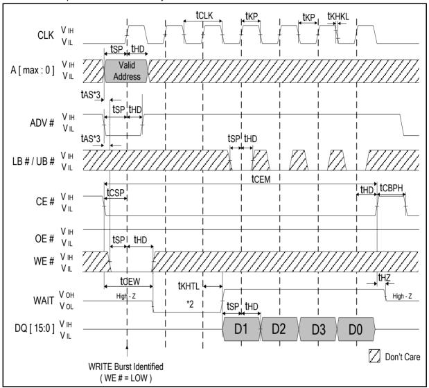
Note: 1. Non-default BCR settings for burst WRITE operation in variable latency mode; Latency code 2)3 clocks); WAIT active LOW; WAIT a asserted during delay; burst length 4; burst wrap enabled.
