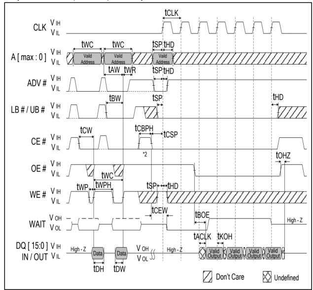
Note: 1. Non-default BCR settings for asynchronous WRITE, with ADV# LOW, followed by burst READ: Fixed or variable latency; latency code 2(3 clocks); WAIT active LOW; WAIT asserted during delay.
