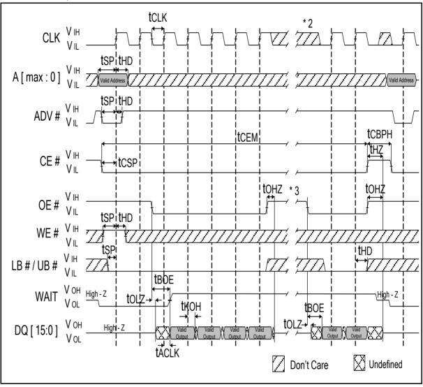
Note: 1. Non-default BCR settings for READ burst suspend; Fixed or variable latency code 2(3 clocks); WAIT asserted during delay.
