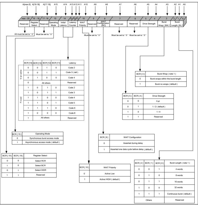
Note: 1. Burst wrap and length apply to both READ and WRITE operations.
