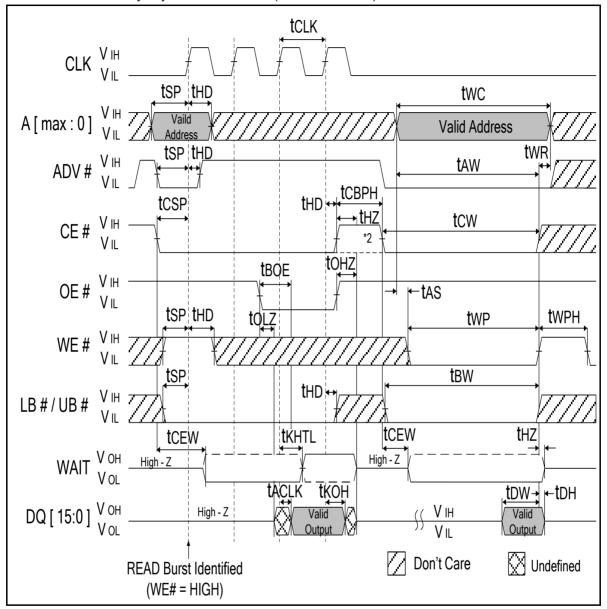
Note: 1. Non-default BCR settings for burst READ followed by asynchronous WE#-controlled WRITE: Fixed or variable latency; latency code 2(3 clocks); WAIT active LOW; WAIT asserted during delay.
