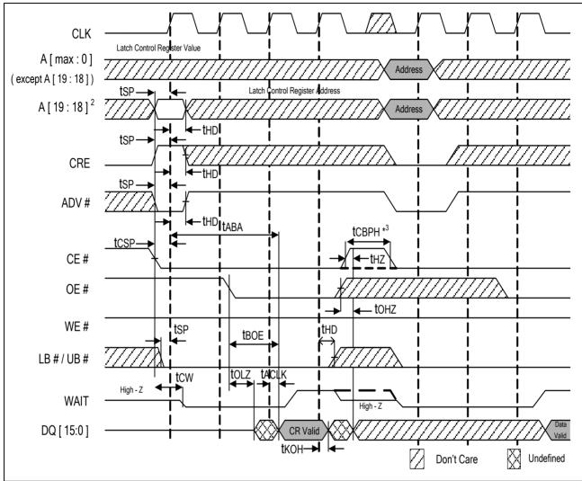
Note: 1. Non-default BCR settings for synchronous mode register READ followed by READ ARRAY operation: Latency code 2 (3 clocks); WAIT active LOW; WAIT asserted during delay.
