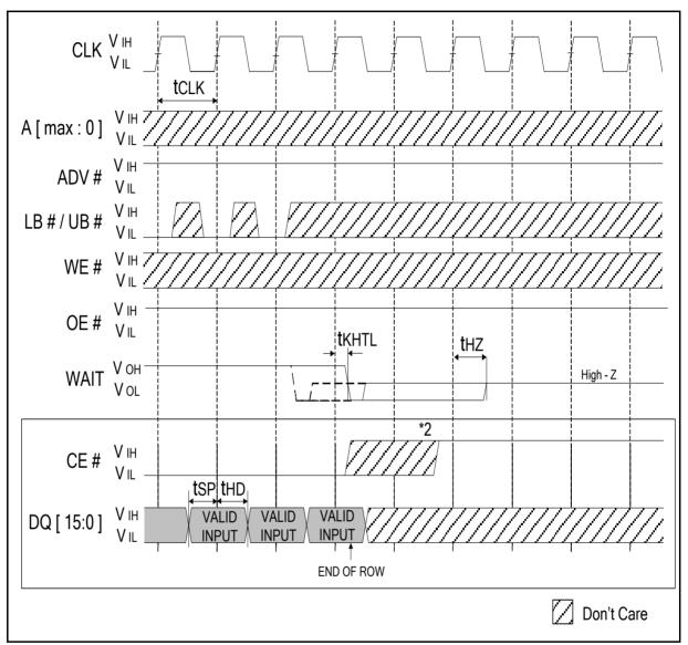
Note: 1. Non-default BCR settings for burst WRITE at end row; fixed or variable latency; WAIT active LOW; WAIT asserted during delay.
