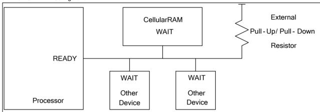
Once a READ or WRITE operation has been initiated, WAIT goes active to indicate that the CellularRAM device requires additional time before data can be transferred. For READ operations, WAIT will remain active until valid data is output from the device. For WRITE operations, WAIT will indicate to the memory controller when data will be accepted into the CellularRAM device. When WAIT transitions to an inactive state, the data burst will progress on successive clock edges.
