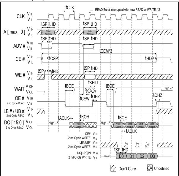
Note: 1. Non-default BCR settings for burst READ interrupted by burst READ or WRITE: Fixed or variable latency code 2(3 clocks); WAIT active LOW; WAIT asserted during delay. All bursts shown for variable latency; no refresh collision.
