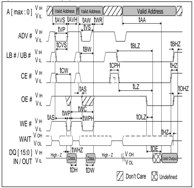
Note: 1. When configured for synchronous mode (BCR[15] = 0), CE# must remain HIGH for at least 5ns (tCPH) to schedule the appropriate refresh interval, Otherwise, tCPH is only required after CE#-controlled WRITEs.
