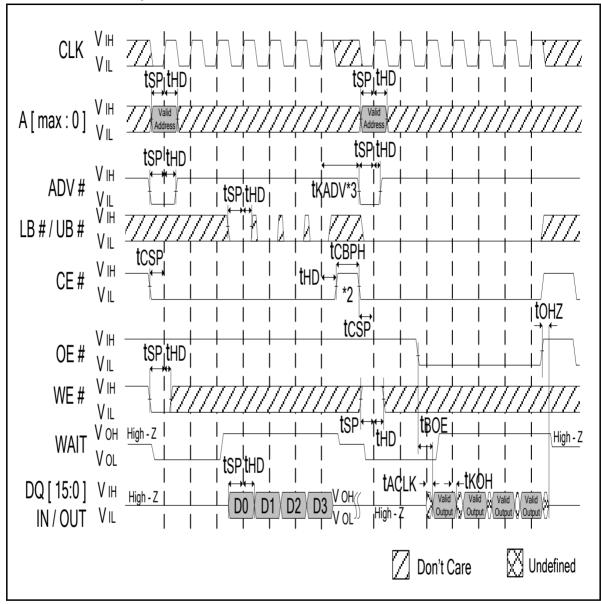
Note: 1. Non-default BCR settings for burst WRITE followed by burst READ: Fixed or variable latency; latency code 2(3clocks); WAIT active LOW; WAIT asserted during delay.
