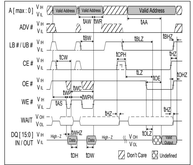
Note : 1. When configured for synchronous mode (BCR[15] = 0), CE# must remain HIGH for at least 5ns (tCPH) to schedule the appropriate refresh interval, Otherwise, tCPH is only required after CE#-controlled WRITEs.
