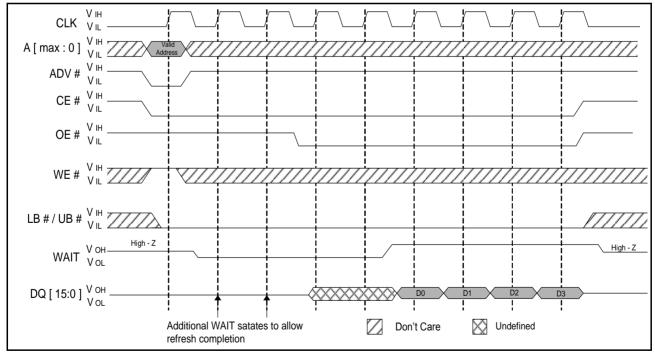
8.2.3.3 Refresh Collision During Variable-Latency READ Operation
