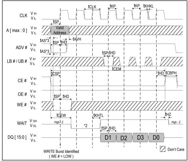
Note : 1. Non-default BCR settings for burst WRITE operation in fixed latency mode; Fixed latency, latency code 2)3 clocks); WAIT active LOW; WAIT a asserted during delay; burst length 4; burst wrap enabled.
