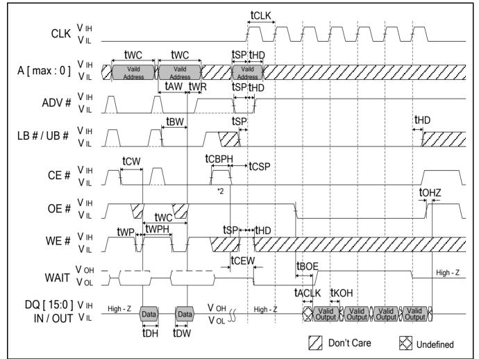
Note : 1. Non-default BCR settings for asynchronous WRITE ,with ADV# LOW, followed by burst READ: Fixed or variable latency; latency code 2(3 clocks); WAIT active LOW; WAIT asserted during delay.
