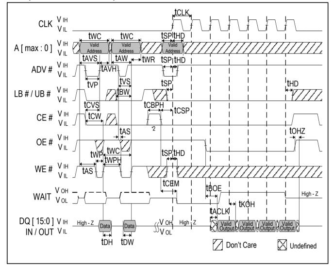
Note : 1. Non-default BCR settings for asynchronous WRITE followed by burst READ: Fixed or variable latency; latency code 2(3 clocks); WAIT active LOW; WAIT asserted during delay.
