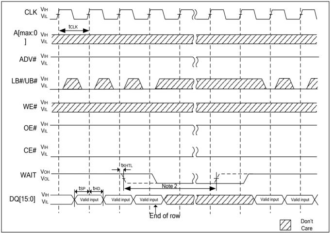
Notes : 1. Non-default BCR settings for burst WRITE at end of row : foxed or variable latency, WAIT active LOW, WAIT asserted during delay (shown as solid line).
