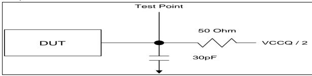
Note: All tests are performed with the outputs configured for default setting of half drive strength (BCR[5:4] = 01b).
