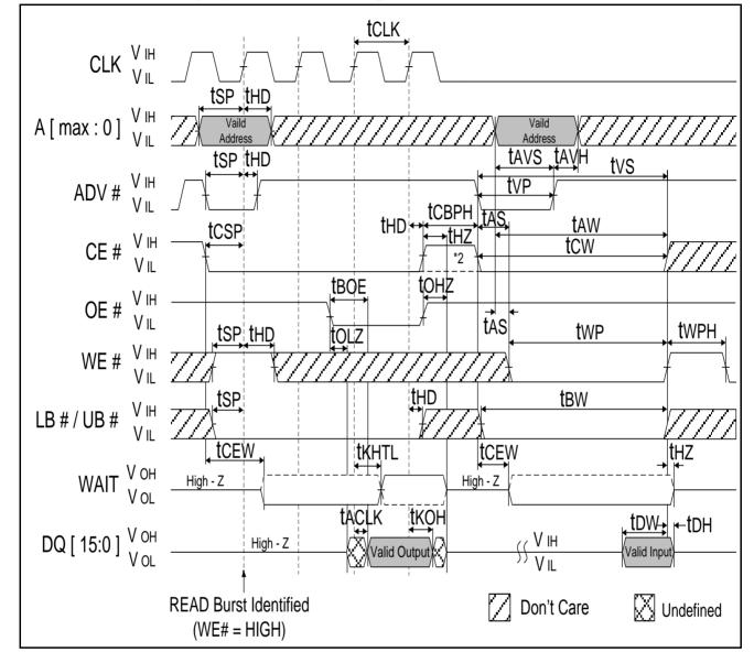
Note : 1. Non-default BCR settings for burst READ followed by asynchronous WRITE using ADV#: Fixed or variable latency; latency code 2(3 clocks); WAIT active LOW; WAIT asserted during delay.
