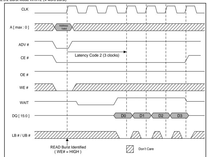
Note : Non-default BCR settings for burst mode WRITE (4-word burst) : Fixed or variable latency; latency code 2 (3 clocks); WAIT active LOW; WAIT asserted during delay.
