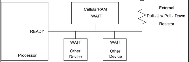
Once a READ or WRITE operation has been initiated, WAIT goes active to indicate that the CellularRAM device requires additional time before data can be transferred. For READ operations, WAIT will remain active until valid data is output from the device. For WRITE operations, WAIT will indicate to the memory controller when data will be accepted into the CellularRAM device. When WAIT transitions to an inactive state, the data burst will progress on successive clock edges.
