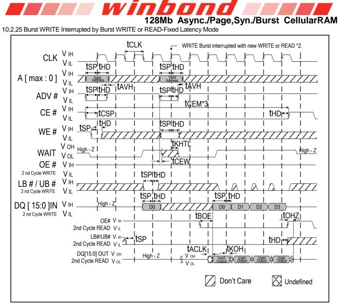
Note : 1. Non-default BCR settings for burst WRITE interrupted by burst WRITE or READ in fixed latency mode: Fixed latency; latency code 2(3 clocks); WAIT active LOW; WAIT asserted during delay.
