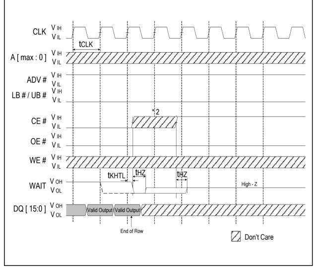
Note : 1. Non-default BCR settings for burst READ at end of row; fixed or variable latency; WAIT active LOW; WAIT asserted during delay.
