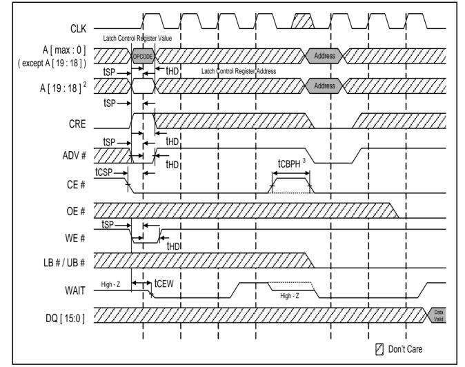
Note : 1. Non-default BCR settings for synchronous mode configuration register WRITE followed by READ ARRAY operation: Latency code 2(3 clocks); WAIT active Low; WAIT asserted during delay.
