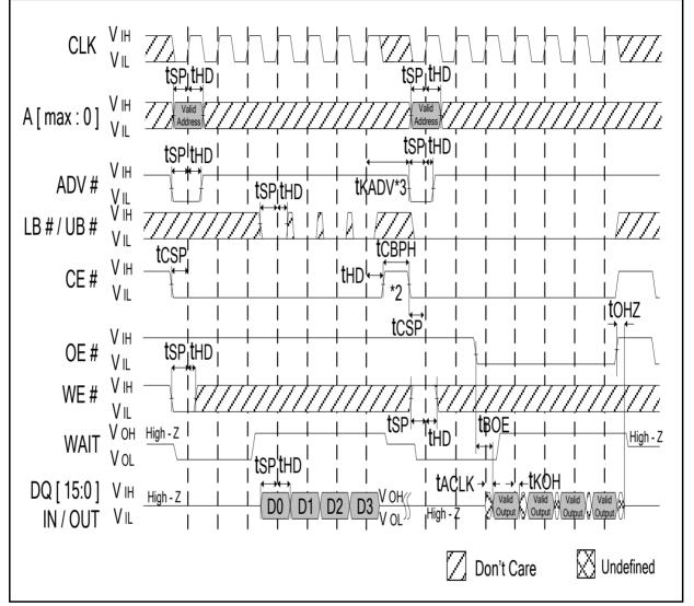
Note : 1. Non-default BCR settings for burst WRITE followed by burst READ: Fixed or variable latency; latency code 2(3clocks); WAIT active LOW; WAIT asserted during delay.
