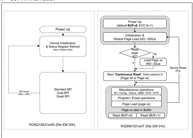
Figure 5. W25M121AV Software Reset Operation Flow
