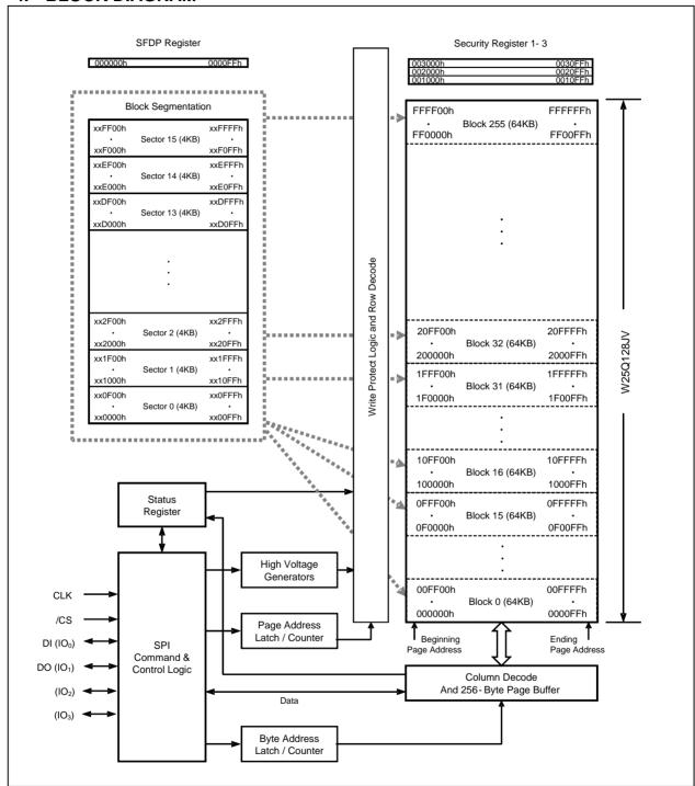
Figure 1. W25Q128JV Serial Flash Memory Block Diagram
