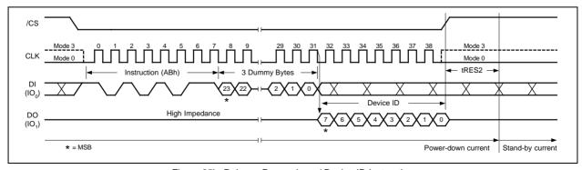
Figure 25b. Release Power-down / Device ID Instruction
