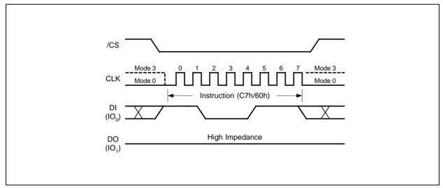
Figure 21. Chip Erase Instruction Sequence Diagram
