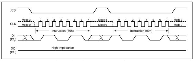
Figure 40. Enable Reset and Reset Instruction Sequence
