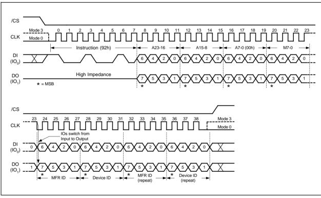
Figure 27. Read Manufacturer / Device ID Dual I/O Instruction
