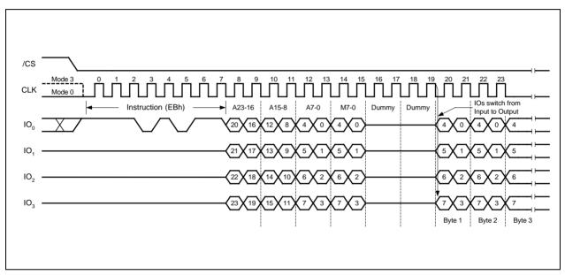
Figure 14. Fast Read Quad I/O Instruction (M7-M0 should be set to Fxh)
