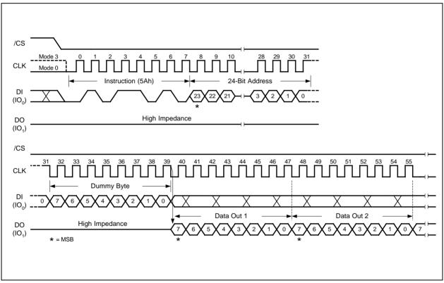
Figure 31. Read SFDP Register Instruction Sequence Diagram
