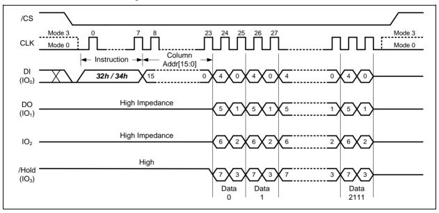
Figure 16. Quad Load / Quad Random Load Program Data Instruction
