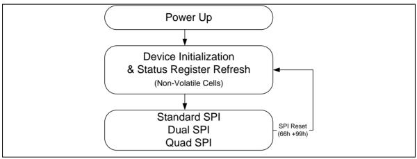
Figure 2. W25Q128JV Serial Flash Memory Operation Diagram
