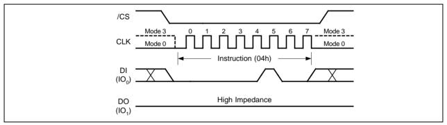
Figure 6. Write Disable Instruction for SPI Mode
