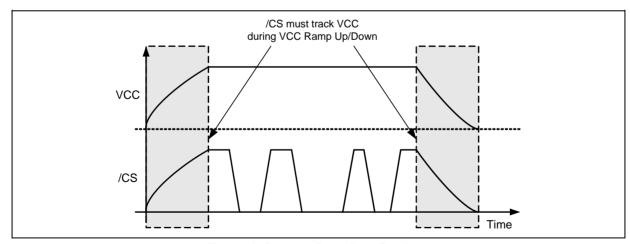
Figure 41b. Power-up, Power-Down Requirement
