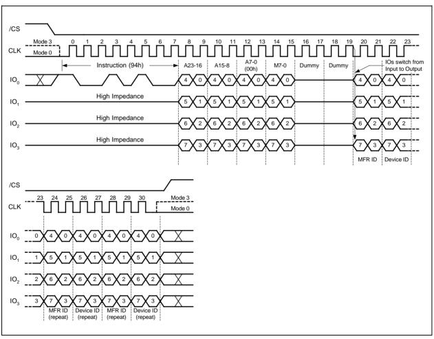
Figure 28. Read Manufacturer / Device ID Quad I/O Instruction
