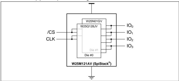
Figure 2. W25M121AV Device Configuration
