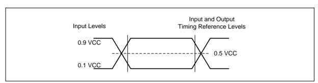
Figure 31. AC Measurement I/O Waveform
