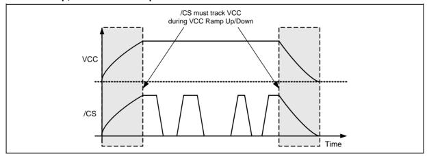
Figure 30b. Power-up, Power-Down Requirement
