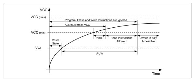
Figure 41a. Power-up Timing and Voltage Levels
