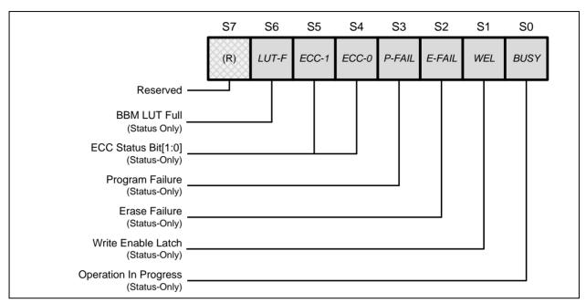
Figure 4c. Status Register-3 (Address Cxh)
