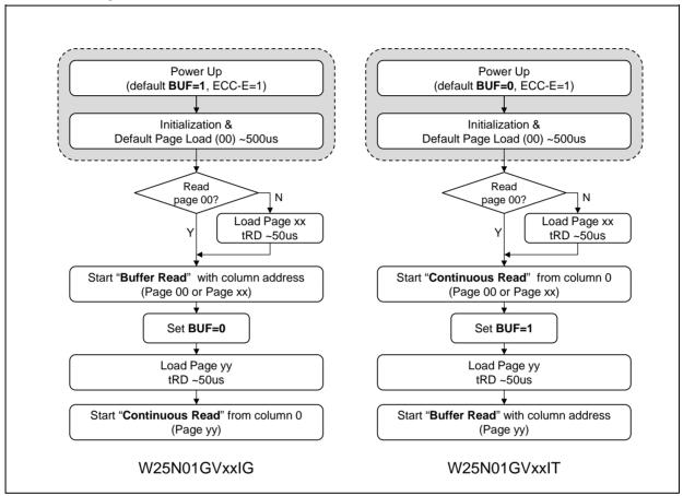
Figure 3. W25N01GV Flash Memory Operation Diagram
