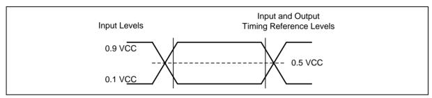
Figure 42. AC Measurement I/O Waveform
