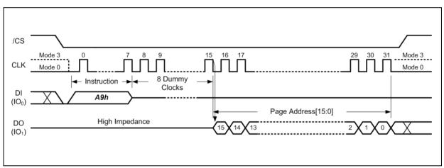
Figure 13. Last ECC Failure Page Address Instruction
