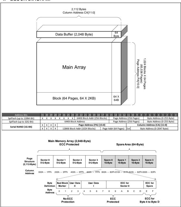
Figure 2. W25N01GV Flash Memory Architecture and Addressing
