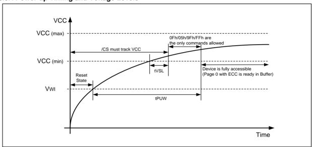
Figure 30a. Power-up Timing and Voltage Levels
