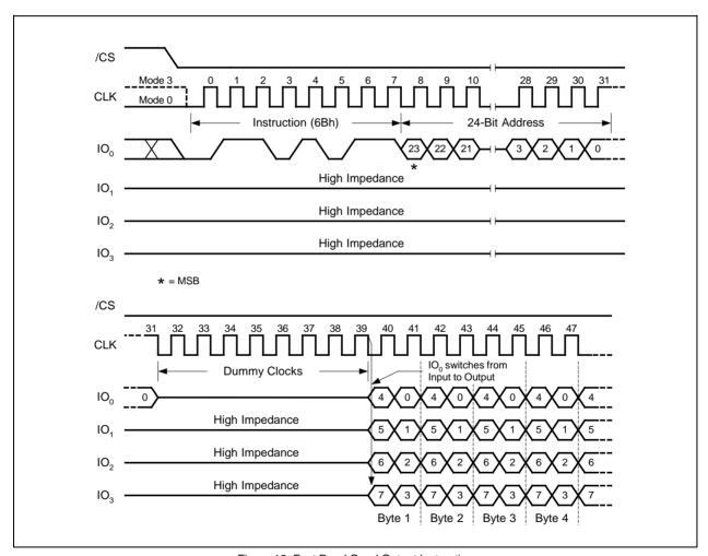
Figure 12. Fast Read Quad Output Instruction
