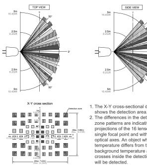
1. The X-Y cross-sectional diagram
