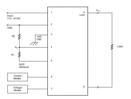
Operate with 5VDC Reference Voltage Variable output
