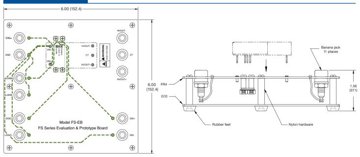
This FS-EB evaluation board provides a convenient package to use any FS Series high voltage power supply without having to it it onto a PC board. The board provides for easy prototyping and evaluation. Please note when ordering, the FS Series unit is not included and must be ordered separately.
