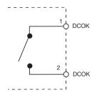
Open = Output fail, if voltage drops below 80% of nominal Closed = Output good
