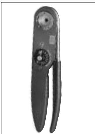
8-Crimp Tool. Adjustable for cross section from 0.38 - 2.5 \text{ mm}^2 (AWG22 - AWG12) Table for adjustment and Contact holder = positioner - see page 46/47
