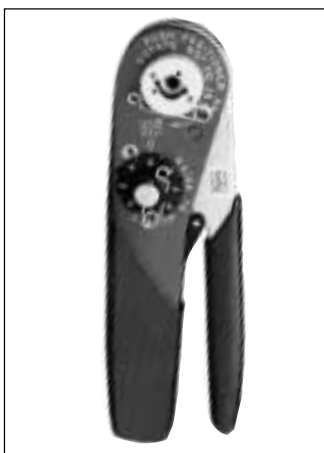
8-Crimp Tool. Adjustable for cross section from 0.08 - 0.5 \text{ mm}^2 (AWG28 - AWG20) Table for adjustment and Contact holder = positioner - see page 46/47
