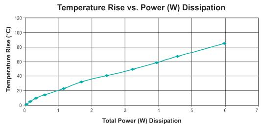
Total Power Dissipation (W) = .001 \* (DCRprimary \* IRMs\_primary<sup>2</sup> + DCRsecondary \* IRMs\_secondary<sup>2</sup>) + Core Loss (W)
