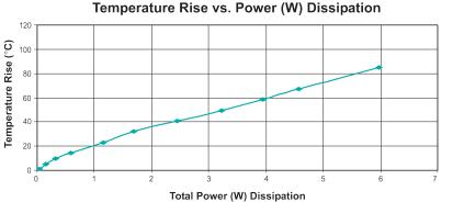
Total Power Dissipation (W) = .001 \* (DCRprimary \* IRMs\_primary<sup>2</sup> + DCRsecondary \* IRMs\_secondary<sup>2</sup>) + Core Loss (W)
