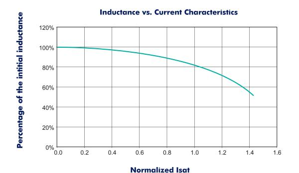
**SMT POWER INDUCTORS** Shielded Drum Core - PL93XX Series Ruggedized
