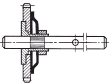
This device is situated inside the gearbox and is particularly recommended when gearbox protection is required in the event of accidental overloading. In this system, the final gear is connected to the gearbox output shaft by means of a friction assembly.
