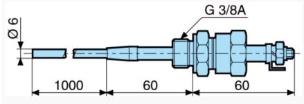
Electrode holder with a single probe supplied in a standard length of 1000mm. (304 stainless steel). Mounting with external 3/8" BSP thread and hexagonal head. Use 24 mm. spanner for hexagon. Suitable for use on boilers, autoclaves and under high temperature conditions up to 200 °C and high pressure conditions up to 25 kg/cm 2
