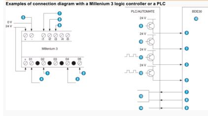
NB : The "tachometer" and "actual direction of rotation" card outputs must be connected to inputs i1 and i2 respectively in order to be able to use the Motomate high-speed counter function.
