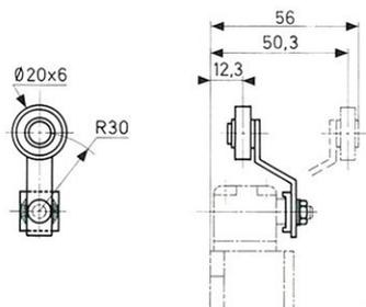
\* Lever settings or positions dictated by direction in which block 1 is fitted (see page 34)
