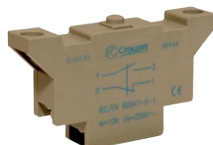
Economic version (839930): SPDT form Za without positive opening, Ø 3.2 mounting holes on top face, screw terminals
