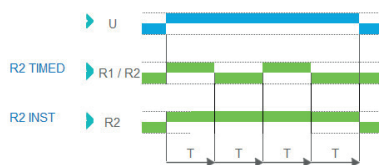
Function Ht - Interval summation time relay
