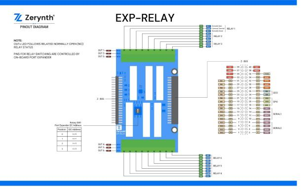
LED: The EXP-RELAY has 6 LEDs. Each relay has a dedicated LED that signals its state.
