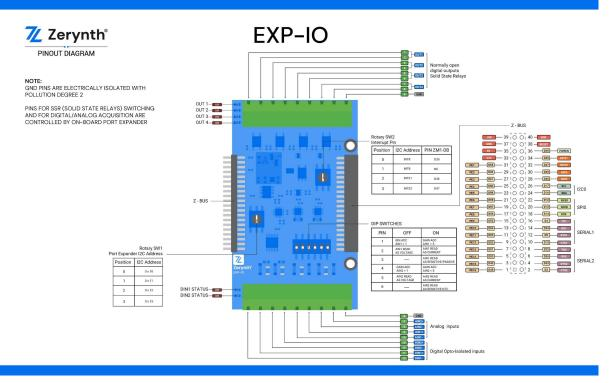
**LED:** The expansion board has 6 pins, each of the 4 relays has a dedicated LED to signal its state. DIN1, DIN2 also have status LEDs.
