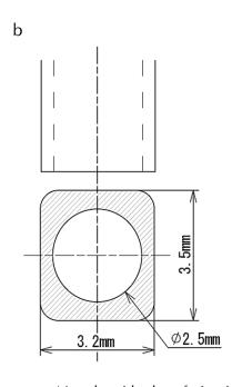
Nozzle with chamfering is recommended
